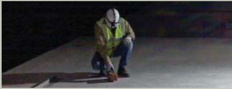
◀ Night-time transmission measurements on bunker roof.
